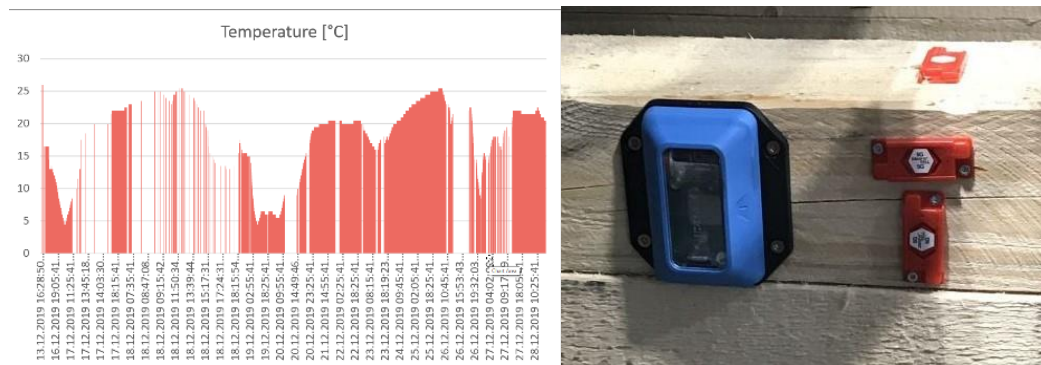
Example of a temperature log profile (left) and real-world application of a data logger at SGL (right)
