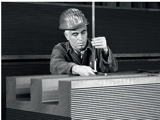
Tolerance testing of graphite cathodes used in aluminum production
