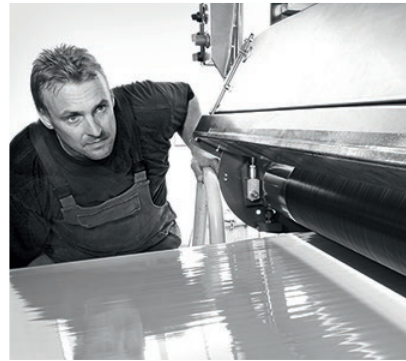
Visual check of prepregs for lightweight components
