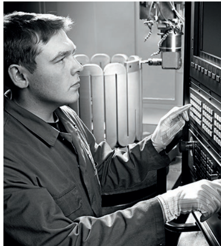
Processing a meander heater made of fine grain graphite for the semiconductor industry
