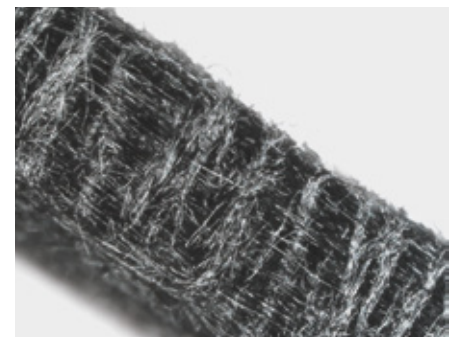
↑ Cross section view of a carbon fiber needle felt
