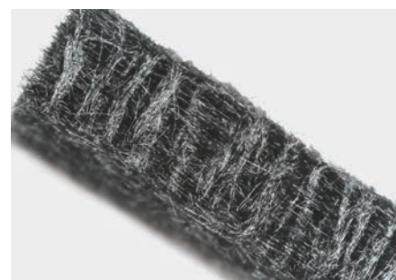
↑ Cross-section view of a carbon fiber needle felt
