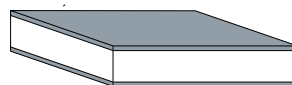
← Protective liners and diffusion barriers – Off-gas from production parts can build up undesired deposits and dendrites or could corrode or oxidize graphite furnace parts. SIGRAFLEX is used as a protective liner on carbon and graphite components like rigid felt resulting in a longer service life.
