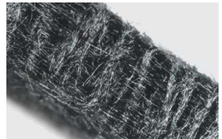
↑ Homogenous fiber structure without gaps and seams
