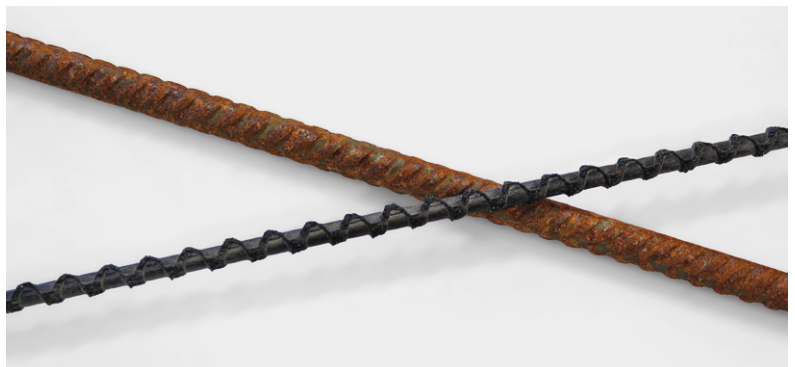
↑ CFRTP rebar with same force at break as depicted steel solution
