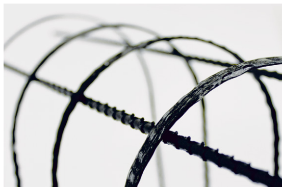
↑ CFRTP reinforcement cage
