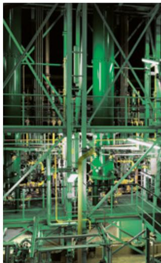
↑ Bottom-fired synthesis unit mounted in skid
