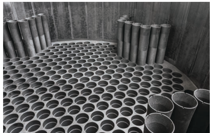
↑ DIABON quencher DN2700 with selected pipes installed
