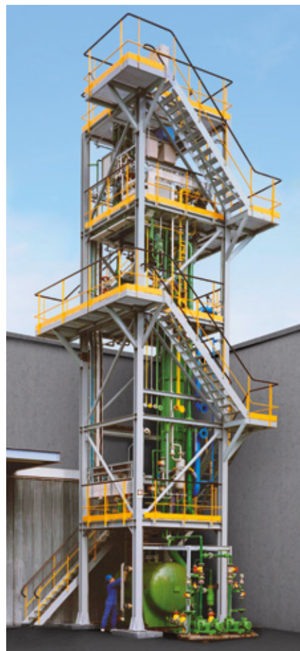
↑ Skid-mounted, top-fired HCl synthesis
