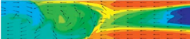
**Original operation point:** the CFD analysis revealed that the original operating point caused inhomogeneous swirling flow resulting in precipitation on the product. Velocity vectors (arrows) and temperature distribution (contours) in the oven plane illustrated above.
