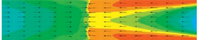
**Optimized operating point:** with the CFD model it is possible to test different operating conditions in a short timeframe. In the optimized operating conditions, we systematically identified the ideal setting for the six inlet flaps and three outlet flaps controlling the gas fluxes and temperatures. The result is a homogeneous in-plane velocity for improved product quality and significant energy savings.
