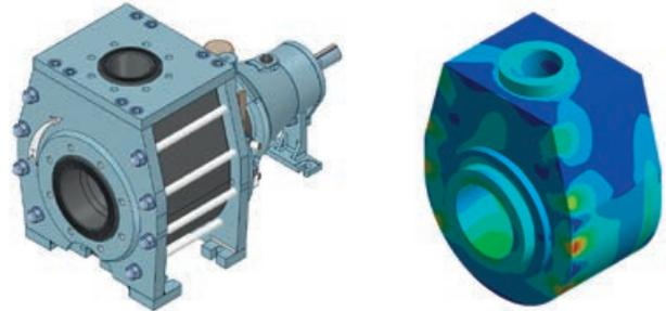
The obtained shape was smoothed and prepared for 3D printing using CARBOPRINT Si material in a binder-jetting process. In the final post-processing step, the 3D printed carbon was infiltrated with liquid silicon to form a ceramic carbon composite material with ideal properties for harsh environments and high temperatures.
