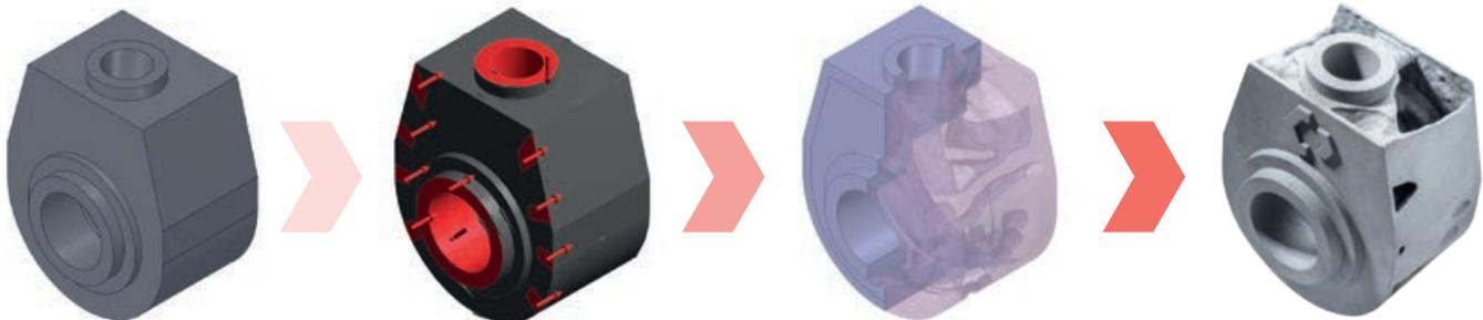
**Digital process chain for creating radically new designs in extremely short timeframes. Optimized design of pump insert: 35% less material providing the same performance.** The optimization results in radically new shapes that can be realized with additive manufacturing.
