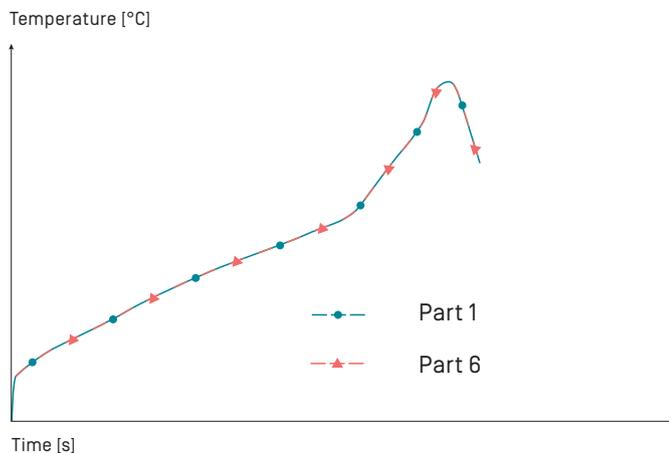
**Temperature curve of different parts subject to optimized firing program:** the dashed and dash-dotted lines show the temperature curve of parts 1 and 6, respectively. The overlapping temperature curves indicate a homogeneous temperature distribution throughout the entire firing cycle. This is achieved through the new furnace design combined with an optimized firing program.
