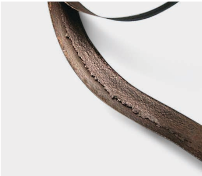
↑ Two photos of a graphite gasket that failed after strong oxidative degradation.
